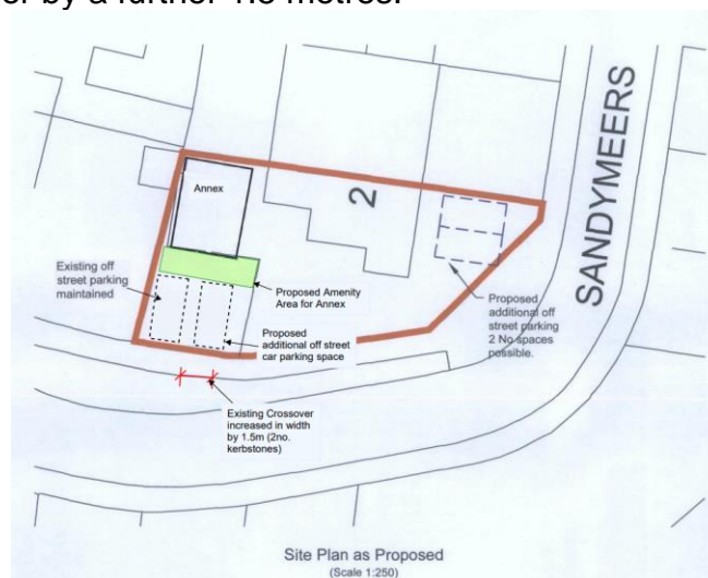
Fig. 2 - Site layout plan showing parking for 2 Sandymeers/Annexe and proposed amenity area for Annex
